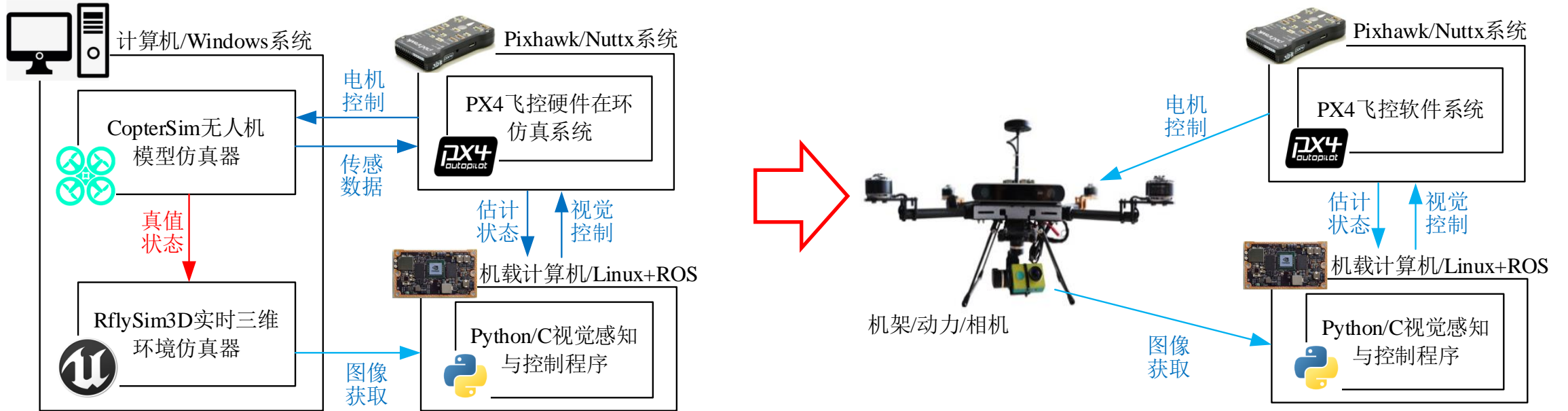
(c) “机架+自驾仪+通信链路+机载计算机” 真机实验
